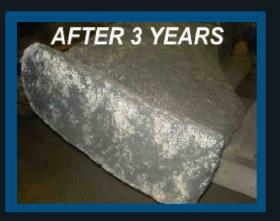
By utilizing our Chesterton ARC-MX-1 reinforced ceramic composites we can rebuild your Ekato mixer blades to exact tolerances which saves downtime on changing out new blades.
